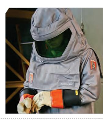
SALISBURY PRO-WEAR® ARC FLASH PERSONAL PROTECTION EQUIPMENT KITS AVAILABLE IN ATPV RATING OF 55 AND 75 CAL/CM<sup>2\*</sup>. These kits contains an arc flash coat, bib overalls, PRO-H00D®, hard hat, SKBAG and safety glasses.
